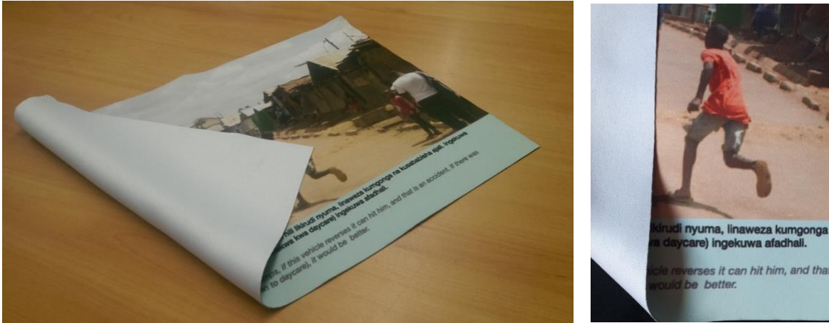
FIGURE 2 – SAMPLE PHOTOS OF ‘BLOCKER’ CLOTH, A THIN, VERY LIGHT WEIGHT, HIGHLY DURABLE POLYESTER MATERIAL WHICH DOES NOT WRINKLE WHEN IT IS PACKED AWAY
